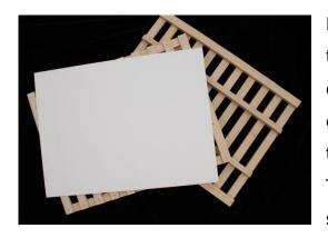
Plant press – In discovering new territory the explorer also encountered new types of plants. They carried plant presses to collect the unknown specimens and take them back to the east for further study. The press consisted of a wooden frame for support, space between the slates for
