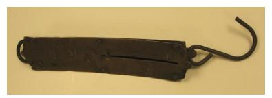
**Scale** – This scale uses a spring and a hook to determine weight. As the weight of an item pulls the hook downward, an indicator
