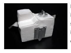
**Display & Control Module** – This is meant to imitate the module astronauts use to operate the systems in their Primary Life Support Subsystem. It is worn on the front of the suit on the astronaut's chest so he or she can reach the controls.
